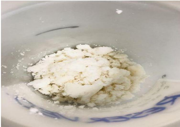
*Figure 6 – Final Filtered 2<sup>nd</sup> Stage LiOH Crystals*
