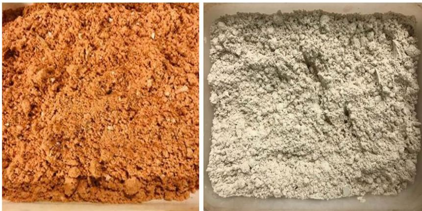
*Figure 4 – Acid roasted calcined spodumene (left) and residual solids after water leach (right)*
