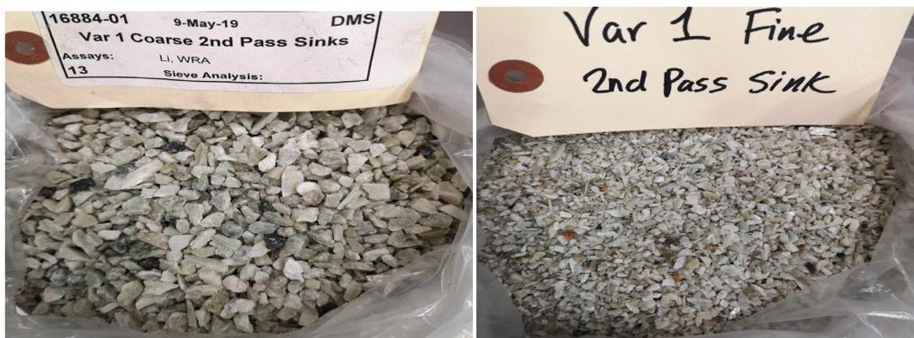
*Figure 1. Coarse and fine final DMS concentrates produced from Piedmont composite samples*
